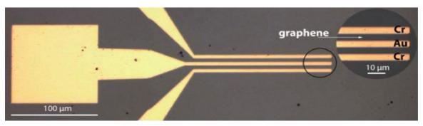
Top-down view of broadband, ultra-fast graphene detector capable of detecting terahertz frequencies at room temperature. (Cr = chromium, Au = gold).
